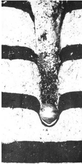
Fig. 4. Section of a cavity in a sand target for penetration of a spherical projectile.
